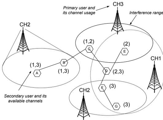
Fig. 1. An example open spectrum system
