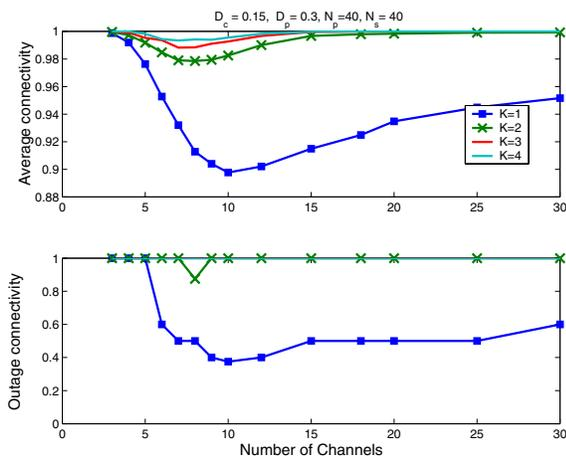
Fig. 8. The ratio of average and outage connectivity corresponding to hash table size  $K$ . The results are based on 1000 random deployment of 40 secondary users, 40 primary users in a  $1 \times 1$  area with  $D_p = 0.3$  and  $D_c = 0.15$ .
