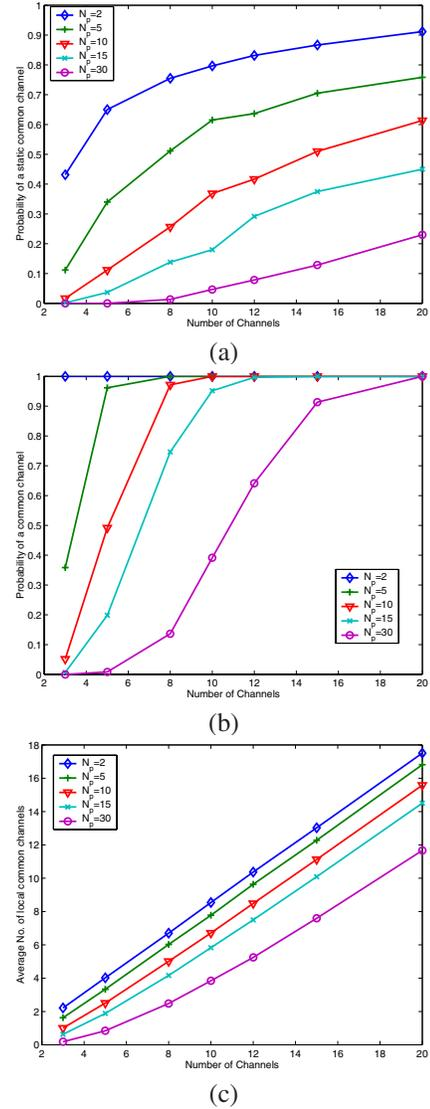
Fig. 2. Statistics of open spectrum systems. Assuming 40 secondary users,  $D_p = 0.3$ ,  $D_c = 0.15$  and 2-30 primary users. (a) The probability of the availability of a predefined common channel among all the users. (b) The probability of the availability of a common channel (not predefined) among all the users. (c) The average number of common channels each user shares with all of its neighbors.
